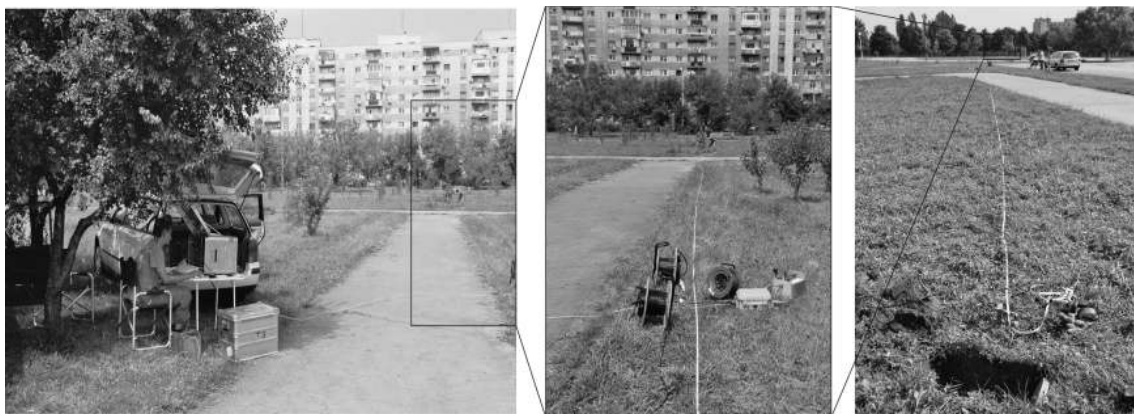
Fig. 3. Measurement in Parc Tineretului; in the hole at the bottom of the right image the inclined steel plate for the generation of the shear waves is visible.
