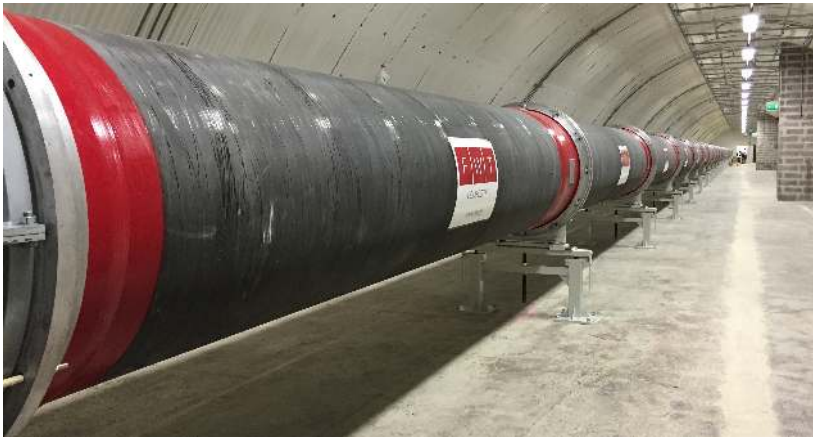
FIGURE 1. Photograph of the 111.5 m long CICLOPE facility with the measurement location seen at the far end.
