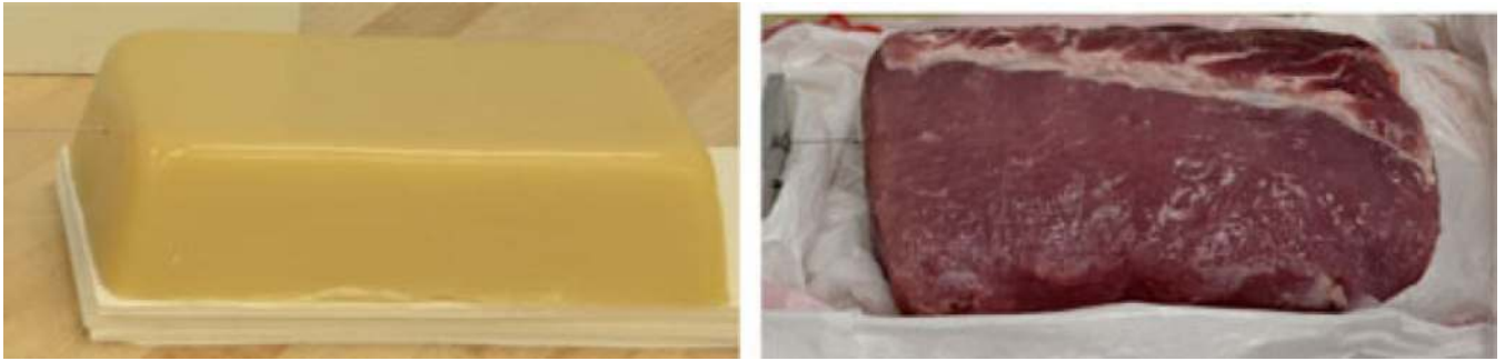
Fig. 7. (Left) Sim-Test tissue phantom. (Right) Porcine tissue ex vivo .
