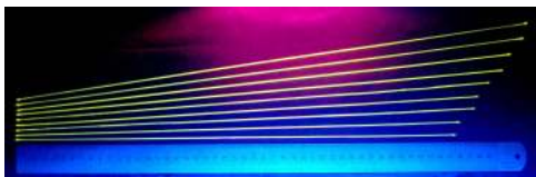
Fig. 9. LuAG:Ce 3+ fibers produced in ILM Lyon using micropulling-down technique.
