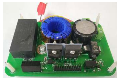
FIGURE 14. Synchronous Boost converter based on TPH3205WS.
