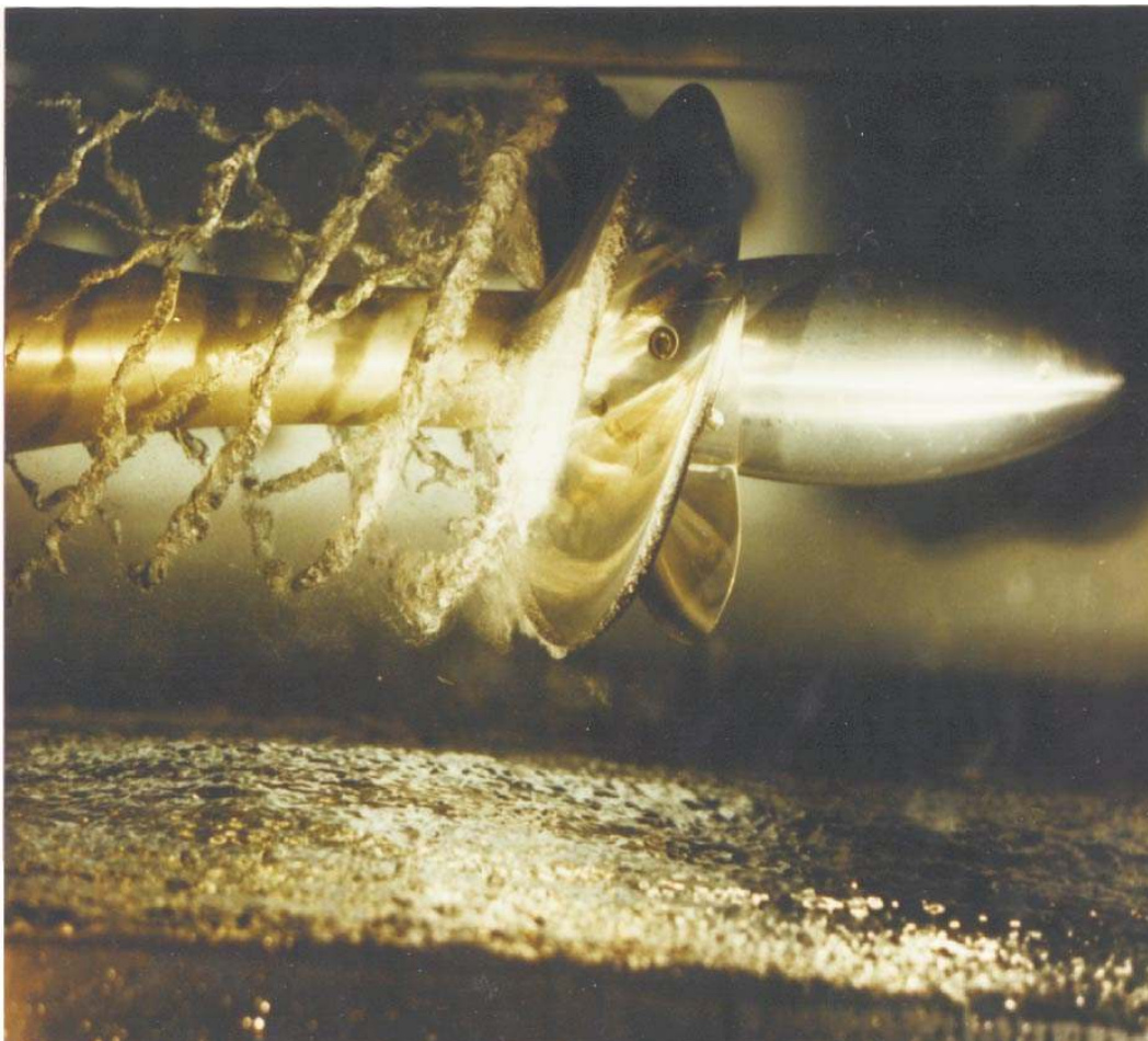
FIGURE 1. VORTEX lines are generated at the edge of boat propellers in motion. Toward the core of the vortices, the liquid velocity increases and the pressure decreases. The lower pressure triggers cavitation, and the resulting bubbles produce noise, vibrations, and erosion of the propellers. (Photo courtesy of DGA-DCE, Bassin des Carenes, Paris, France.)
