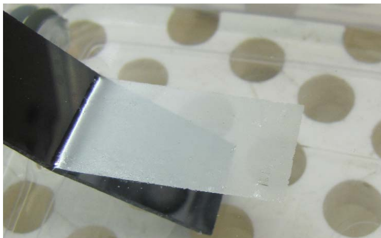
Figure 1. Free-floating laminar metal/dielectric/metal nanomembrane, strata thickness 10 nm + 15 nm + 10 nm, metal Au, dielectric silica, lateral dimensions 2 cm × 8 mm, support polished Si.
