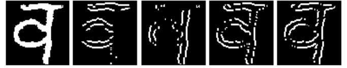
Fig. 5 Four sub-images (right side) obtained using four Kirsch operators (4-7) and fifth sub-image (left side) obtained due to original image, Fig. 4(a), after normalizing its size to 70 \times 70 pixels.
