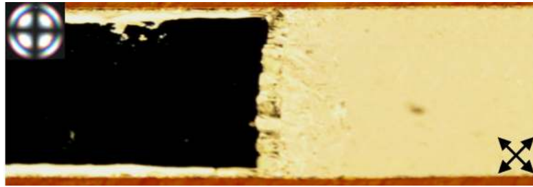
Figure 6.3: Polarized micrograph of a microchannel possessing composite boundary conditions. Shown here: the left half is homeotropic, and right half is uniform planar. Such microchannels can be utilized to produce micro-flows with spatially modulated velocities.
