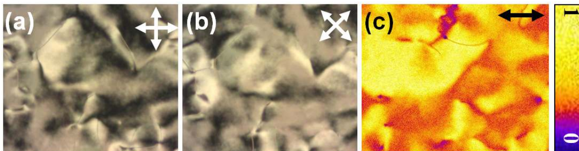
Figure 4.3: LC anchoring on untreated glass surface. (a), (b) Polarizing optical micrographs of 5CB confined in a glass LC cell observed between crossed polarizers at relative orientations of 0 and \pi/4 . (c) Corresponding FCPM micrograph obtained with polarized laser. The polarization state is denoted by the double-headed arrow. The domain structures observed through polarized light and fluorescence intensity distribution indicate random orientations of \vec{n} in the azimuthal plane of the cell (degenerate planar anchoring). Colour intensity of 1 and 0 respectively correspond to molecular orientation parallel and perpendicular to the laser polarization in (c).
