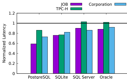
Figure 9: Latency of test query plans created by Neo after 100 episodes of training, normalized to plans created by the target system’s corresponding optimizer for different workloads.
