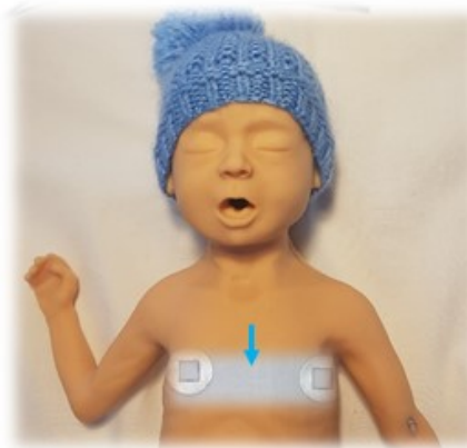
Fig. 2. Close-up view of the EPS sensor front-end showing a see through view of the silver deposited electrodes (blue arrow).
