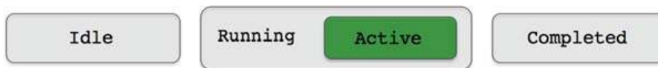
Figure 9. Behavior states: A behavior may be in one of these four states at any given iteration of the helm Iterate() loop. The state is determined by examination of MOOS variables stored locally in the helm's information buffer.
