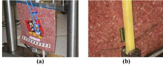
Fig. 7. In vitro characterization with soft tissue in (a) front view showing antennas and (b) back view showing the sensor.
