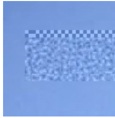
Figure 2: Appearance of the synchronization and the actual watermark patterns for a high embedding strength ( s=10 )
