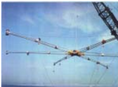
Fig. 1. NESTOR detector floor showing the two detector modules at the end of each of the six support arms, the central electronics housing and modules.
