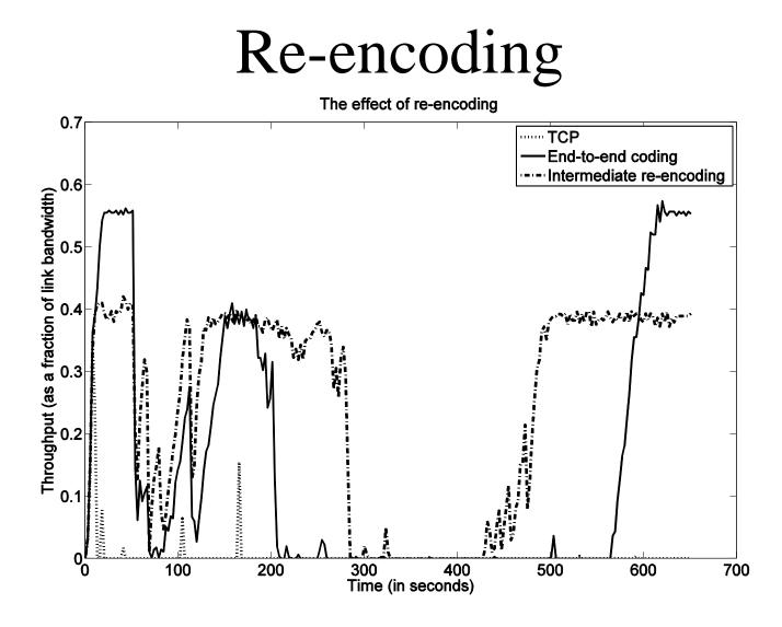
TCP: 0.0042 Mbps; Coding E-to-E: 0.1420 Mbps; Re-encoding: 0.2448 Mbps
