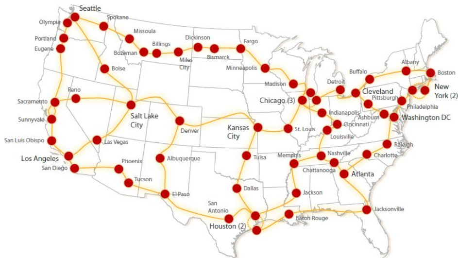
Fig. 5. Draft of the planned U.S. UCAN network using the Internet2 100G deployment. (Source: [112]).
