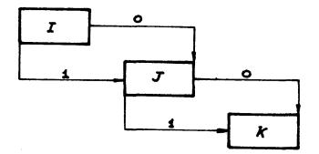
Using the first method, we assume, that I, J and K have durations of exactly 5, 3 and 4 days respective. We represent the results of the calculations by means of a Gantt-chart.
