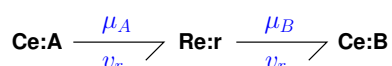
Figure 3: Bond graph of the reaction A \rightleftharpoons B . \mu_A is the chemical potential associated with the chemical species Ce:A , \mu_B is the chemical potential associated with Ce:B and v_r is the molar flow associated with the reaction Re:r .
