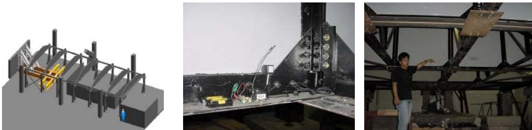
Figure 7. Test apparatus (a) sketch (scale indicated by person in lower right), (b) instrumentation, and (c) structural assembly (indicates high-degree of redundancy in structure)
