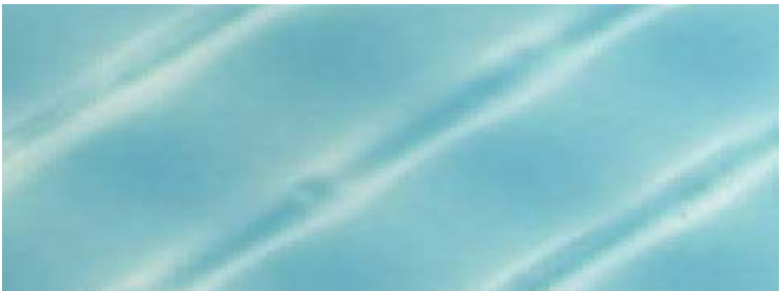
Fig. 10-13 Visualization of mass transfer distribution for spacers with a constant inclination angle \phi , \phi = 45^\circ , \lambda = 4-11 , 0.5% METHOCEL ® K15M, Re_M = 10 .
