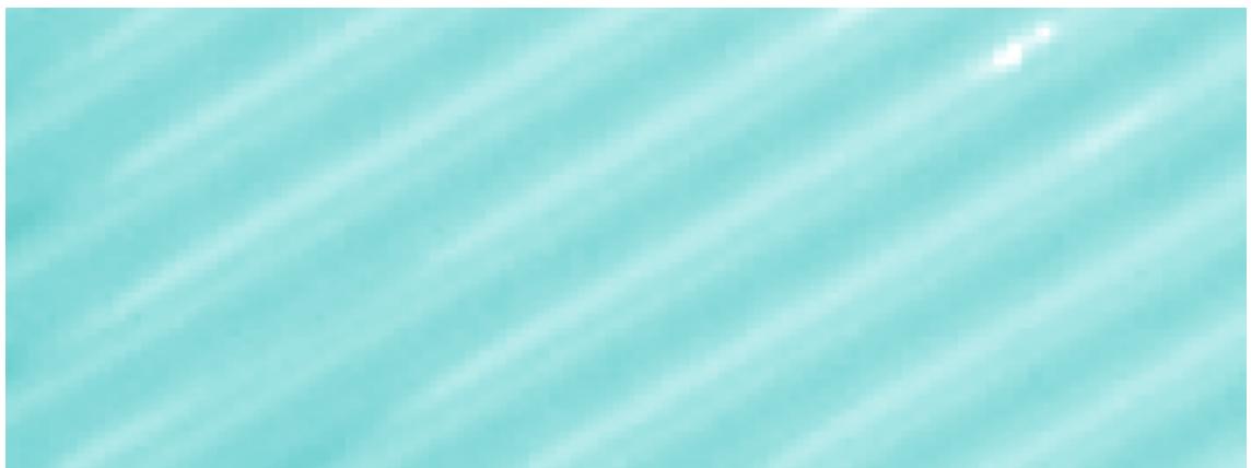
Fig. 10-12 Visualization of mass transfer distribution for spacers with a constant wavelength, \lambda/a = 4 , \varphi = 15-60^\circ , 0.5% METHOCEL ® K15M, Re_M = 10 .
