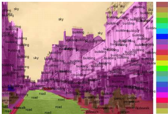
Figure 5. Street scene parsing: a convolutional network was trained on the LabelMe spanish dataset [26] with a method similar to [12]. The training set only contains photos from spanish cities; the image above is a picture taken in Edinburgh. The convolutional network is fully computed on neuFlow, achieving a speedup of about 100x (500x375 images are processed in 83ms, as opposed to 8s on a laptop).
