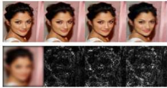
Fig. 6. Reconstruction comparison on the CelebA dataset for the deblur plus noise problem. While the Neumann networks (NN) and gradient descent networks (GDN) perform well, the differences are most apparent the residual images in the second row, especially in the background reconstruction. Residuals are formed by displaying the norm across color channels of the error at each pixel, scaled by a factor of 6.
