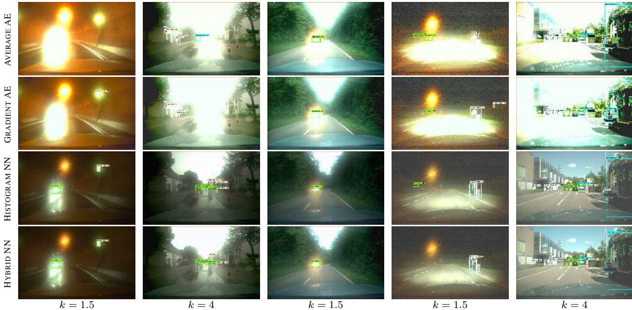
Figure 5: Comparison of the two proposed methods and the two baselines, see text, using simulations of mild ( k = 1.5 ) and moderate ( k = 4 ) exposure shifts.
