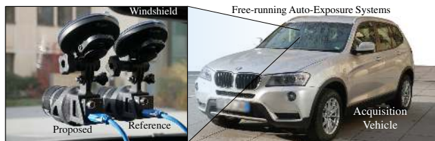
Figure 7: Side-by-side capture setup for the experimental comparison of the proposed Hybrid NN with the average-based auto-exposure control baseline, see text.
