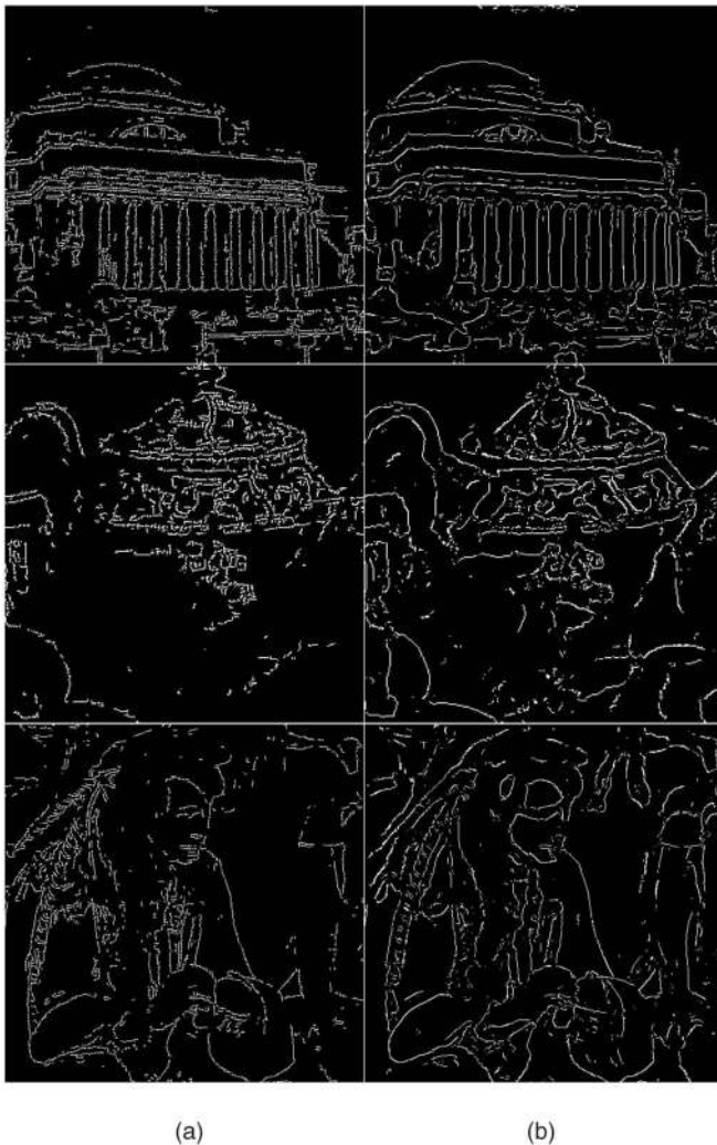
Fig. 16. Comparison of edge detection of the NEE with that of a leading edge detector for natural images with constant additive white Gaussian noise. (a) Edges detected by the NEE with the edge localization method. (b) Edges detected by the Elder edge detector.
