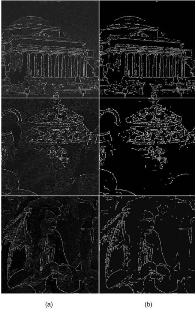
Fig. 14. Results of the detection of edge locations by use of the proposed edge localization method (applies to the edges enhanced by the NEE where the target edge enhancer is the Sobel filter). (a) After nonmaximum suppression. (b) After hysteresis thresholding.
