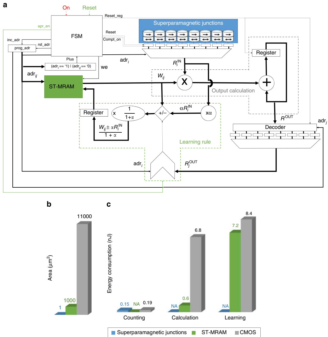
Fig. 5 Design of the full system for the gripper task. a Schematic illustrating the data path of the designed system, associating CMOS circuits, superparamagnetic tunnel junctions, and stable magnetic junctions used as MRAM. (FSM finite state machine, WE write enable, ADR address). b Circuit area occupied by the superparamagnetic tunnel junctions, CMOS, and MRAM. c Energy consumption of the superparamagnetic tunnel junctions, CMOS, and MRAM required to perform one system operation: running the junctions, computing the output, and adjusting the weight. The system has 128 inputs and 128 outputs
