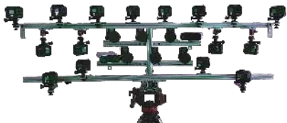
Figure 2. Our custom camera array comprising 16 GoPro HERO7 and 6 central Back-Bone H7PRO cameras (large circular lenses).
