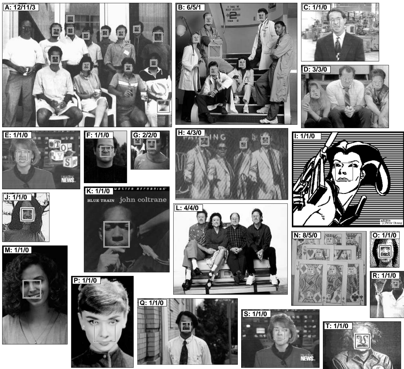
Figure 3: Output obtained from System 11 in Table 1. For each image, three numbers are shown: the number of faces in the image, the number of faces detected correctly, and the number of false detections. Faces are missed in A and H (for unknown reasons), B (large angle), and N (the stylized faces are not reliably detected at the same locations and scales by the two networks, and so are lost by the AND heuristic). False detections are present in A and B. Although the system was trained only on real faces, hand drawn faces are detected in I and N. Images A, H, K, and R were scanned from printed photographs, B, D, G, I, L, and P were obtained from the World Wide Web, C, E, and S are digitized television images, F, J, M, and Q were scanned from photographs, N and T were provided by Sung and Poggio at MIT, and O is a dithered CCD image.
