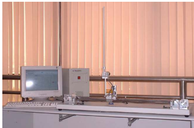
Figure 1.5: PID-like neural network controller, double inverted pendulum system [10]
