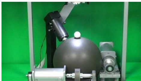
Figure 1.3: Approximate feedback linearization approach, ball-on-sphere system [5]
