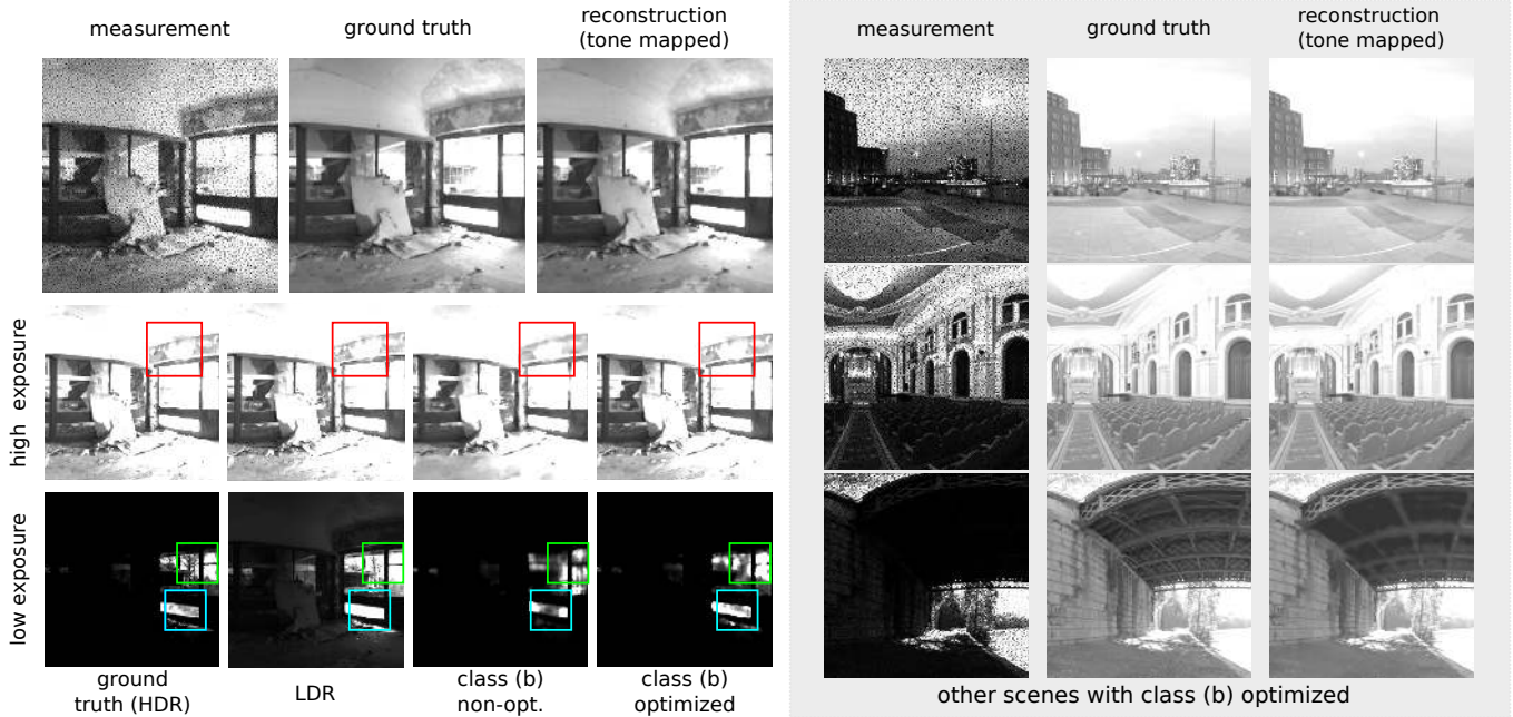
Fig. 5. HDR results in simulation. On the right pane: the images show ground truths, measurements and reconstructions for different HDR scenes captured with shutter functions of class (b) in simulation along with some baseline comparisons. The left pane shows other scenes captured with optimized shutters of class (b).
