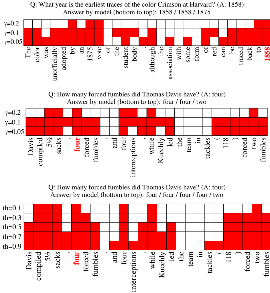
Figure 10: Reading (red) and skimming (white) on SQuAD, with LSTM+Attention model. The top two are skimming models with different values of \gamma . The bottom one is skimming models with different values of skim decision threshold (whose default is 0.5). An increase in \gamma and a decrease in threshold lead to more skimming.
