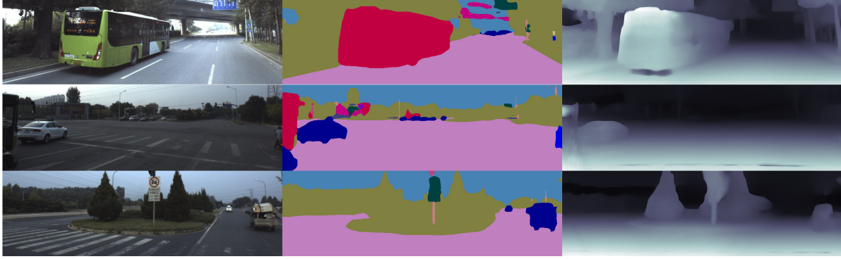
Figure 1: Examples of DNN-predicted segmentation maps (center column, using method [85]) and depth maps (right column, using method [2]), on the Apolloscape dataset [32]. The left column contains the respective RGB image inputs fed to the trained DNNs.
