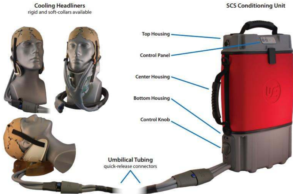
Figure 2. The WElkins Sideline Cooling System used in this study. The conditioning unit contains the top housing (control panel and battery tray), center housing (heat exchanger and ice cartridge housing), and bottom housing (hydraulic and pneumatic components) sections.
