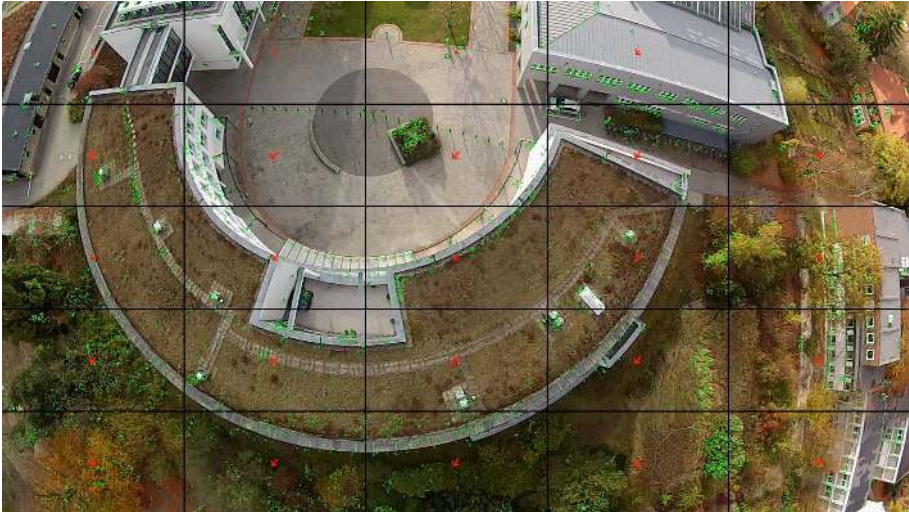
Fig. 5. This figure shows a camera frame captured in-flight over the Institute of Computer Science at Free University Berlin. The frame is overlaid with optical flow features (green points) and average flow vectors (in red) in each of the 25 image bins.
