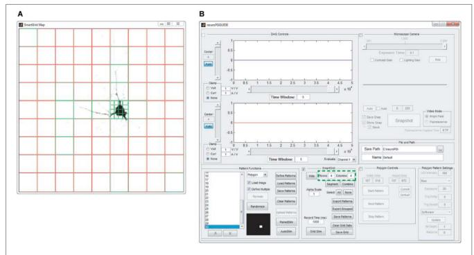
**FIGURE 3** | **SmartGrid pattern generation**. A grid of ROIs is generated based on user-defined grid dimensions (number of rows and columns—highlighted in panel **(B)**) and the grid is overlaid on an image of the field of view to be stimulated, as in panel **(A)**. SmartGrid can
