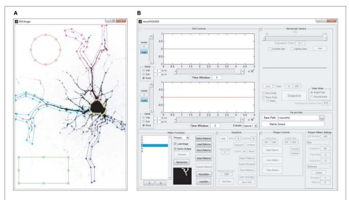
**FIGURE 2 | Manual pattern generation**. ROIs are manually defined as overlays on an image of the field of view that will be stimulated. **(A)** Screenshot of circular, rectangular and spline ROIs, manually defined
