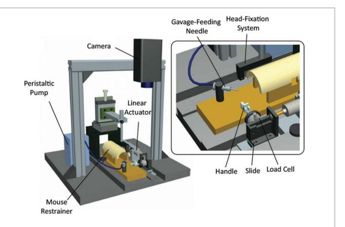
FIGURE 4 | M-Platform for training and measuring motor performance of mice forelimb. Schematic of the robotic device. The main components are indicated: head fixation system, peristaltic pump with a gavage-feeding needle for liquid reward delivery, restrainer, linear actuator, camera to record forelimb position, plastic handle for the retraction task, linear slide and load cell for forces detection. Modified from Spalletti et al. (2014).
