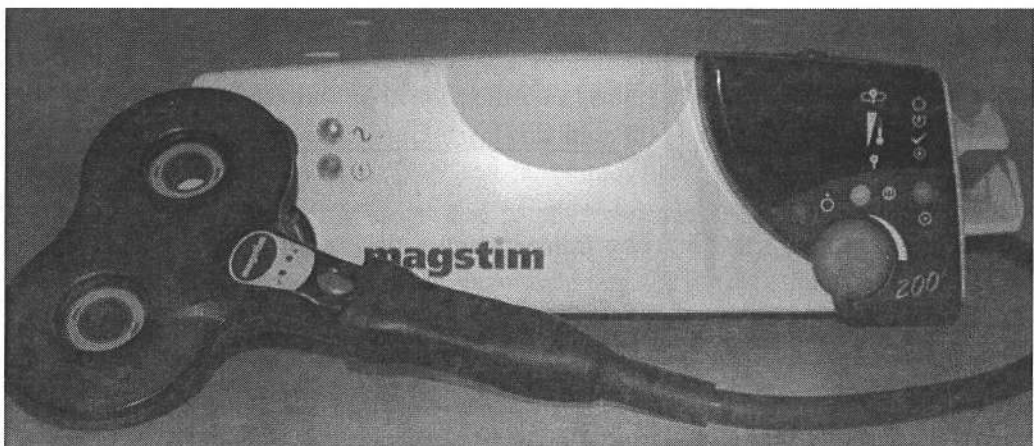
Figure 1. Magstim 200 2 single pulse stimulator with a 'figure of eight' magnetic coil. The figure of eight coil contains two small magnets in reverse polarity enabling a more focused electromagnetic impulse than the standard circular coil (from author's own image collection).
