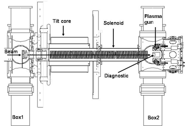
Fig.4: A sketch of compression and neutralization section.
