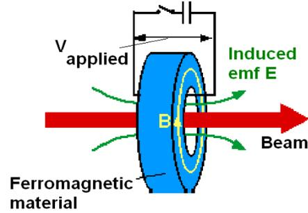
Fig. 3: Schematic of an induction accelerator module.
