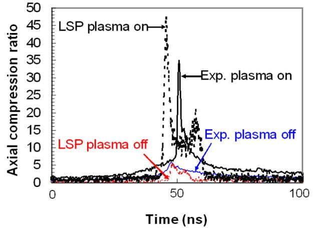
Fig. 12: Experimental data and LSP simulation of beam compression with neutralization (plasma source on) and without neutralization (plasma source off).
