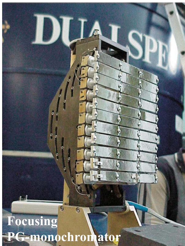
Fig. 10. A vertically focusing PG monochromator used at the Canadian Neutron Beam Centre.
