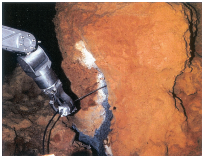
FIG. 2. Loihi hydrothermal vent site. A temperature probe is being inserted into the vent orifice; note the extensive deposits of Fe oxides surrounding the vent opening.
