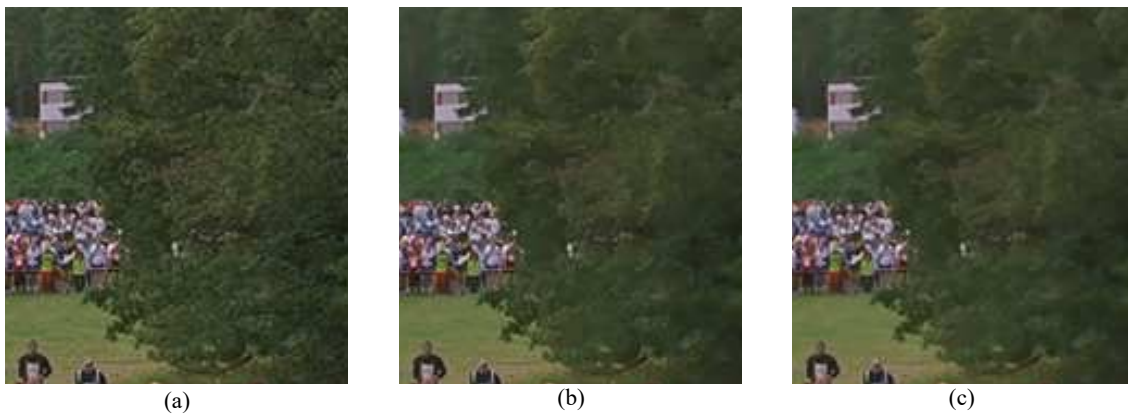
Figure 17. Comparison of quality between a frame of the sequence CrowdRun encoded at QP22 without pre-filter (39.11dB) (a), with TBil(11x11, JND) ( PSNR_{frame} = 36.14\text{dB} , CMOS_{sequence} = -0.50 , BitrateSaving_{sequence} = 9.51\% ) (b) and BilAWA(11x11, JND) ( PSNR_{frame} = 34.84\text{dB} , CMOS_{sequence} = 0.19 , BitrateSaving_{sequence} = 15.66\% ) (c)
