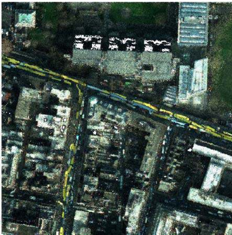
Fig. 1. By letting pixel values be the color value of the highest point in each pixel, a false color orthophoto can unintentionally be generated. Detecting building outlines from such an image is challenging. In this case, the thin rectangles lined end to end are bus roofs. Herein the pixel size represents an area of 0.25 \text{ m}^2 , and the image dimensions are 500 by 500 pixels.
