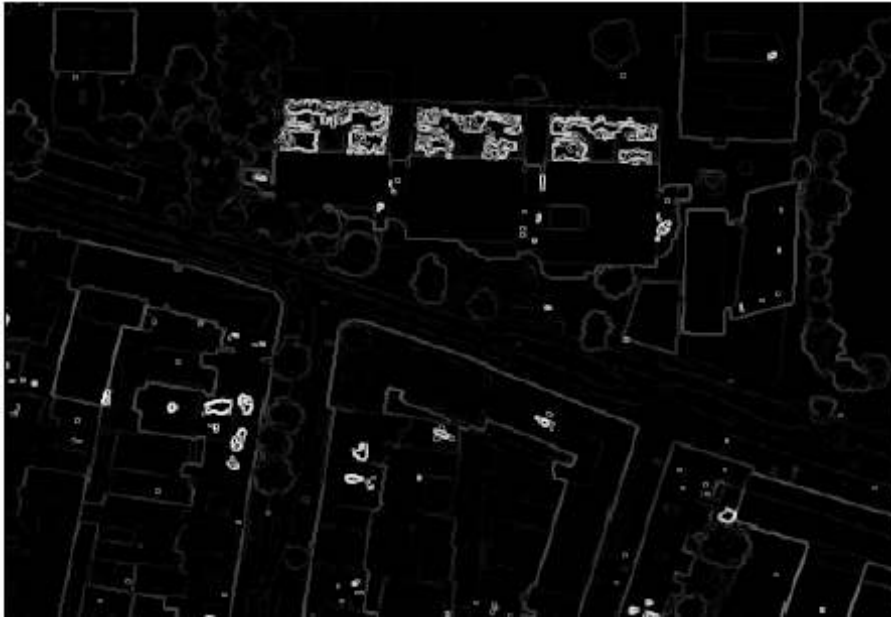
Fig. 4. Derived building outlines by using height threshold.
