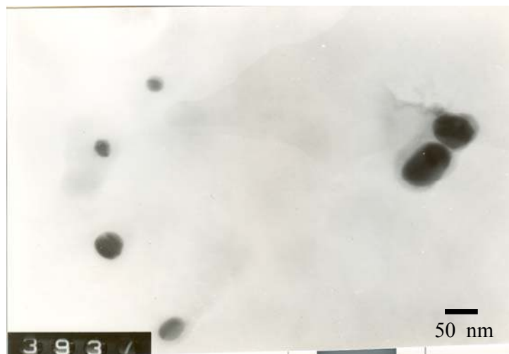
Fig. 3.21 SEM image of the gold nanoparticles after dialysis.
