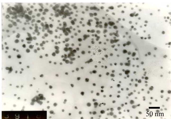
Fig. 3.20 TEM image of the gold nanoparticles before dialysis.
