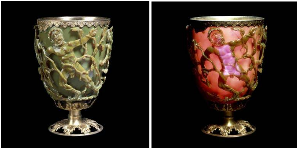
Fig. 1.2 Lycurgus Cup (a) green color, if light source comes from outside of the cup (b) red color, if the light source comes from inside of the cup.
