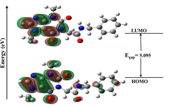
**Figure 13.** The FMO analysis; HOMO and LUMO at the ground state of the molecule at B3LYB/6-311 + +G(d,p).
