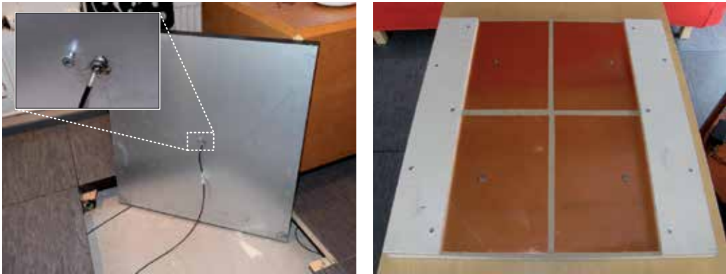
Figure 3. Two different types of tiles with different sizes of electrodes were used as transmitters in the implemented test systems of publications [48], [50], and [51]. The left-hand side of the figure shows the bottom surface of a standard, commercial 60 \times 60 -cm raised floor tile from the TUT Smart Home . The inset photo shows a snap fastener soldered to the middle of the electrode for cable connection and a screw drilled next to it to prevent the snap fastener from being flattened. The right-hand side of the figure depicts a custom-built floor tile with four roughly 30 \times 30 -cm copper foil transmitting electrodes. These electrodes are partly hidden by the two plywood boards on the sides that stiffen the tile and raise it to the same height as the commercial raised floor tiles. [51]
