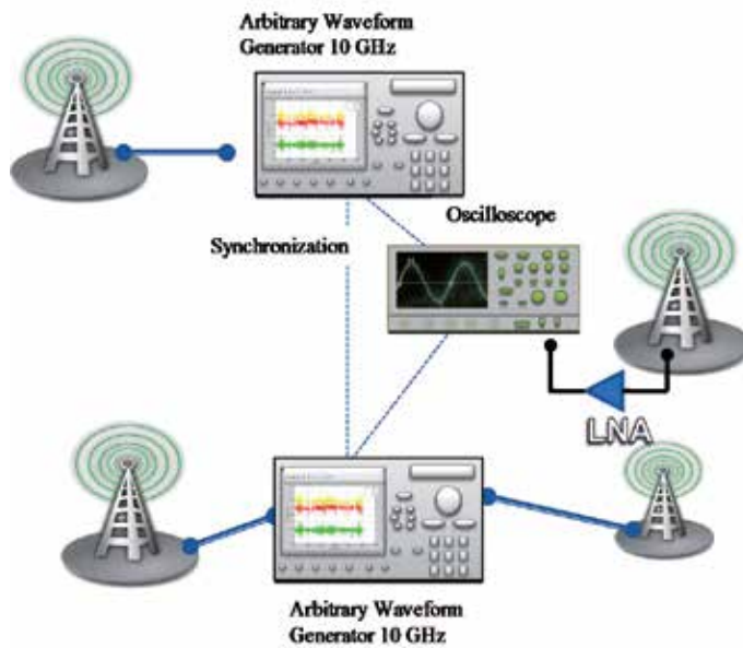
Figure 15. Experimental setup for indoor positioning system.
