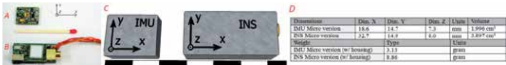
Figure 12. The comparison of the proposed INS (b) with the World's smallest IMU (a). The measurement axes are drawn in the image. c) The comparison of the mounting's size of the presented INS and IMU, d) The comparison of the external characteristics of the proposed INS and the IMU.
