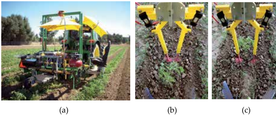
Figure 16. A RTK-GPS based robotic cultivation system-(a) A cultivator retrofitted with a RTK-GPS system in operation, and (b) The cultivating tines open to protect the plant based on the plant map and closed to rid of weeds in between plants in the crop row.
