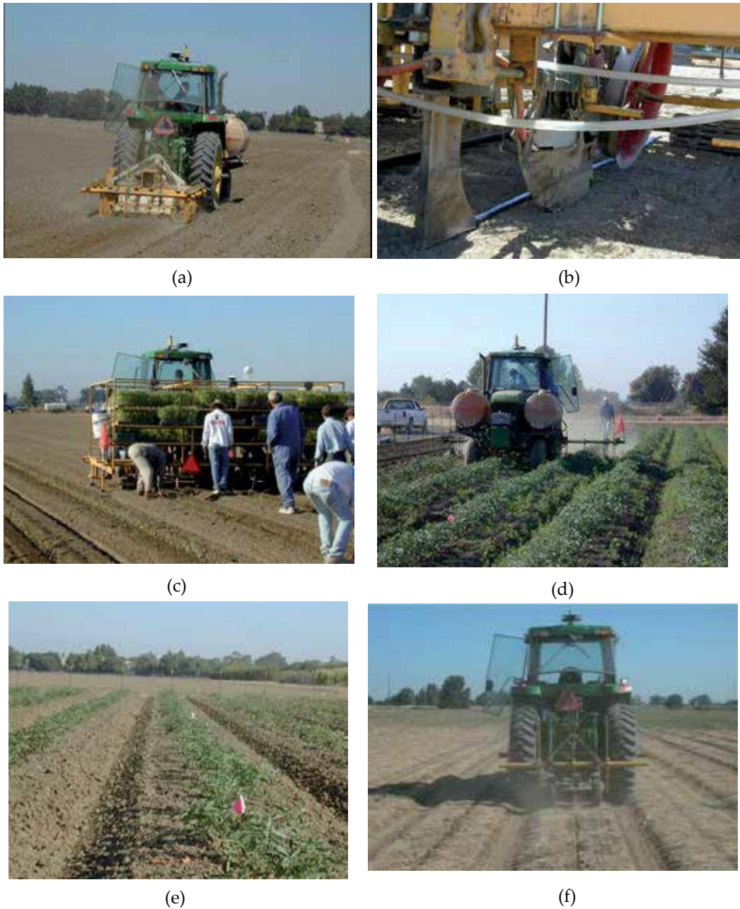
Figure 12. RTK GPS based autoguidance system used for various cultural operations – (a) bedding, (b) drip tape installation setup, (c) transplanting processing tomatoes, (d) cultivation, (e) plants following cultivation, and (f) deep tillage after plant removal.
