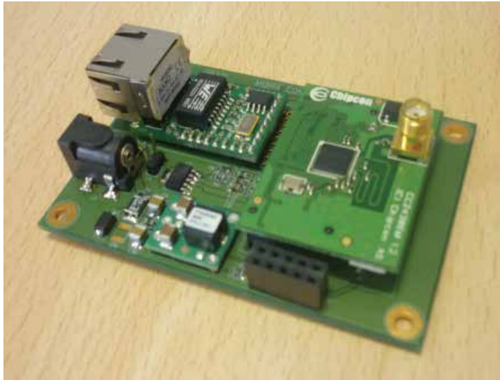
Figure 5. Node main board. The CC2430, the Ethernet module, the power plug and the I/O pins are visible.
