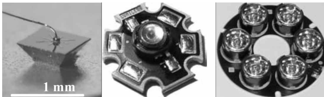
Fig. 2. Light emitting diode (LED) samples: microchip, LED in a package and ring array of LEDs
