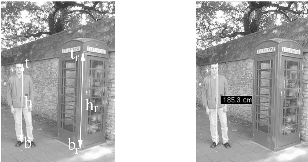
Figure 5. A reference height: (a) The known height of the phonebooth ( h_r ) is used as a reference to measure the height ( h ) of the person standing nearby. t and t_r are top points respectively of the unknown height and of the reference height; b and b_r are the corresponding base points on the ground plane. (b) The height of the person in the picture is measured at h = 185.3\text{cm} . The ground truth height is 187\text{cm} . The discrepancy between measured height and ground truth is caused by the person leaning down slightly on his right leg (see section 5).
