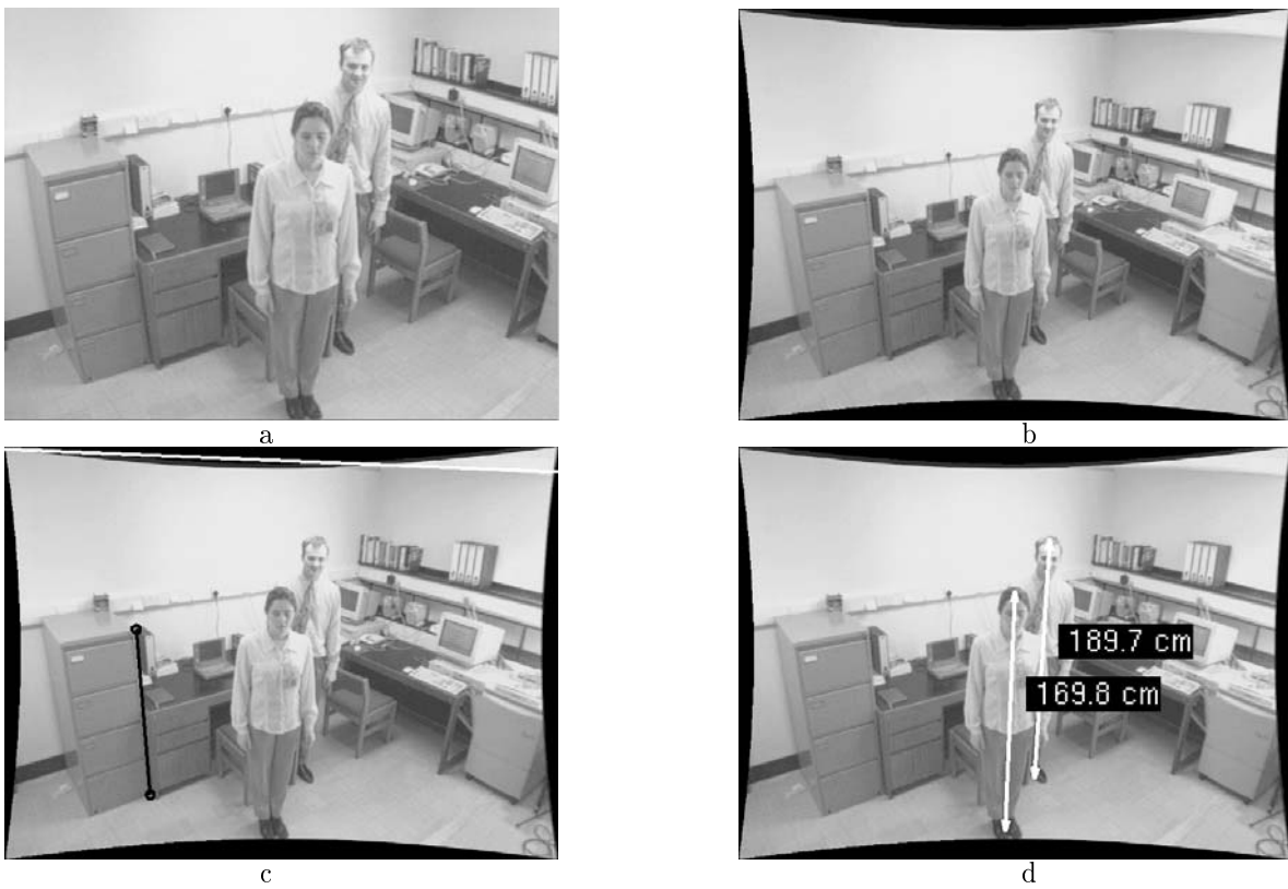
Figure 8. (a) Original image. (b) Image after correction for radial distortion. (c) Vanishing line (in white) and reference height (in black), the filing cabinet is 132\text{cm} high; (d) Height measurements computed from the image. The ground truth is h = 1.90\text{m} for the man and h = 1.70\text{m} for the woman. The computed height of the camera is 2.35\text{m} .
