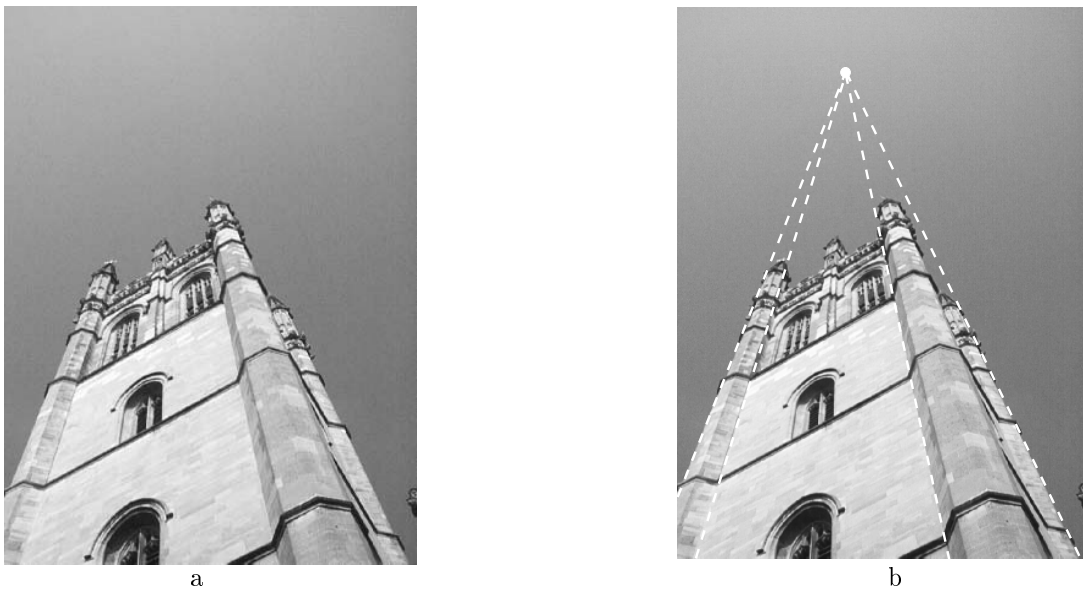
Figure 4. The tower of Magdalen College, Oxford. (a) Original image. (b) All vertical lines intersect in the image plane at the vertical vanishing point, which is marked in white.
