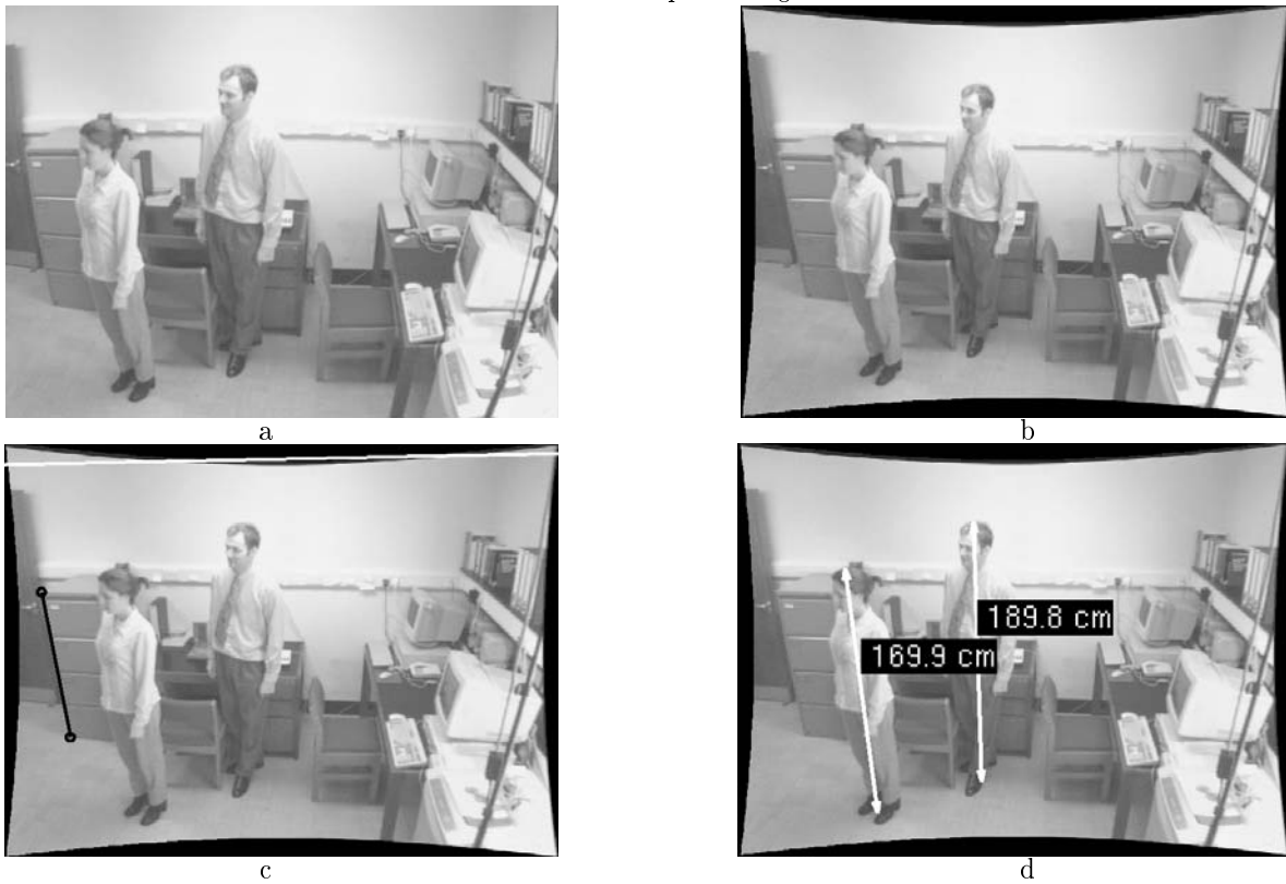
Figure 9. (a) Original image. (b) Image after correction for radial distortion. (c) The vanishing line (in white) and reference height (in black), the filing cabinet is 132\text{cm} high. (d) The height measurements computed from the image. Compare with figure 8. The height of the camera, which is at a different position to that of figure 8, is here computed as 2.24\text{m} .
