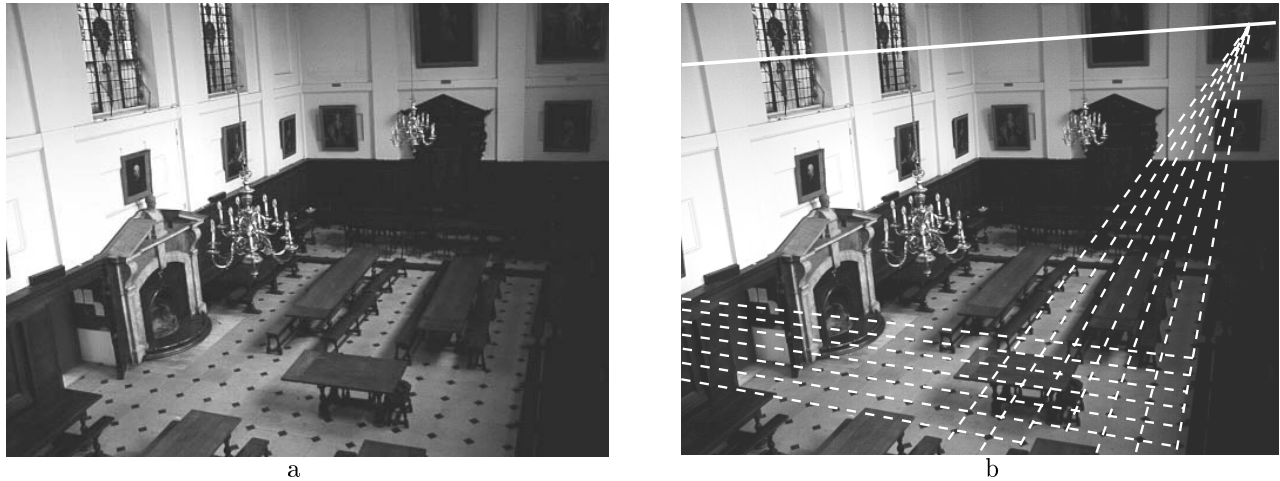
Figure 3. The dining hall of Queen's College, Oxford. (a) Original image. (b) The vanishing line of the floor is shown in solid white; sets of parallel lines on the floor (dashed) intersect in points on the vanishing line.
