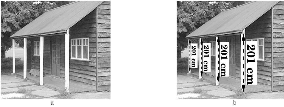
Figure 1. An example of measuring heights from a single image. (a) The four columns have the same height in world, although their images clearly are not of the same length due to perspective effects. (b) As shown, however, all columns are correctly measured to have the same height.
