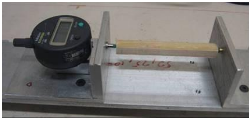
Figure 2.11 Jig for length measurement with a sample inserted in two tubular ends that locate the map pins
