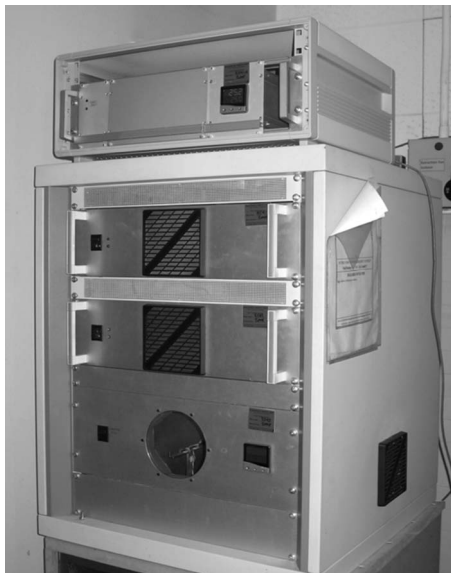
Fig. 10. Environmentally controlled test chamber.
