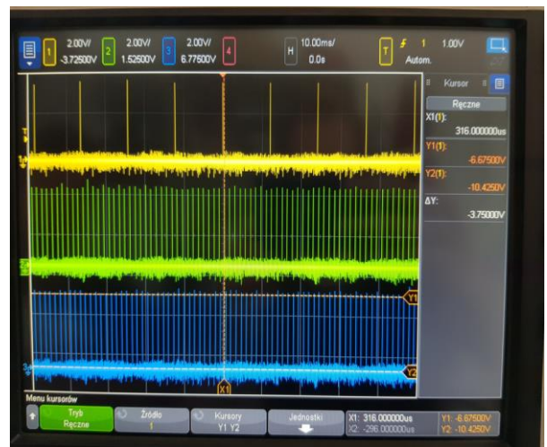
Fig. 7. Signals generated by turbine simulator: 'once per revolution' (yellow) and two blade sensor impulses (green and blue).
